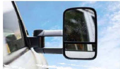
Original Towing Mirrors are much larger than any standard mirror and feature a huge single mirror above a smaller convex mirror - for serious towing!
